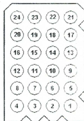
24 pin connector Left Side Wall to Robot's ribbon cable
