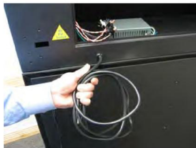
Figure 8b – Undo tie wraps
