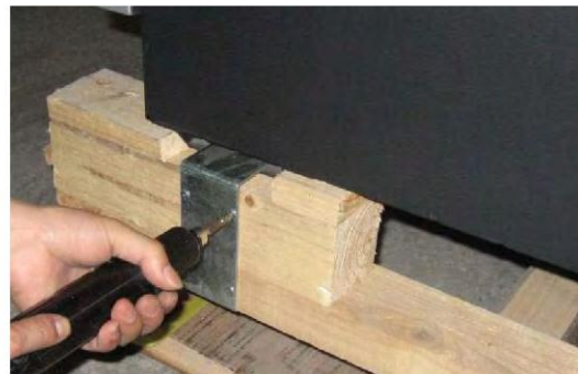
Figure 3– Remove angled brackets
