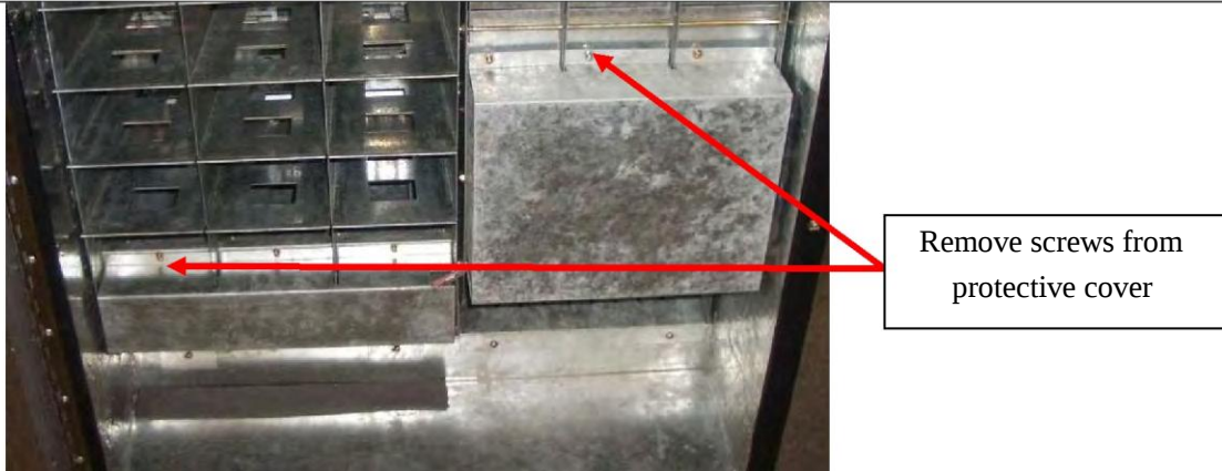
Figure 49 – Remove protective cover
