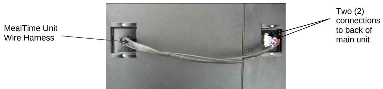
Figure 23 – Wire Harness connection
