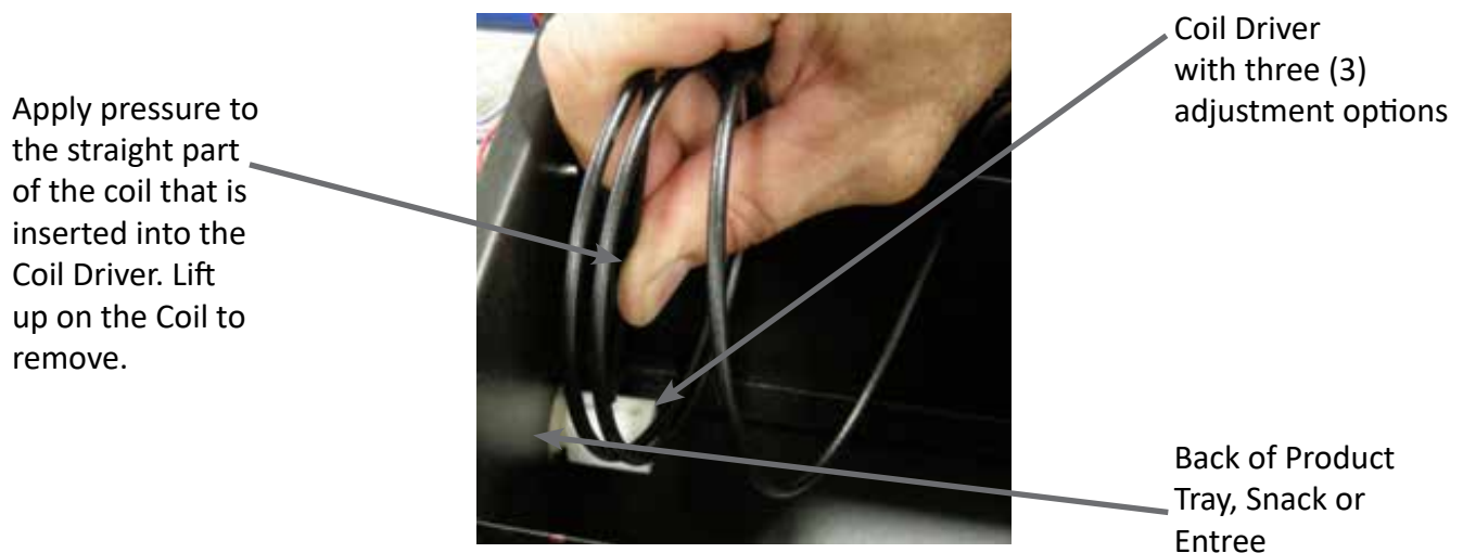
Figure 9 – Removing and Aligning a Coil
